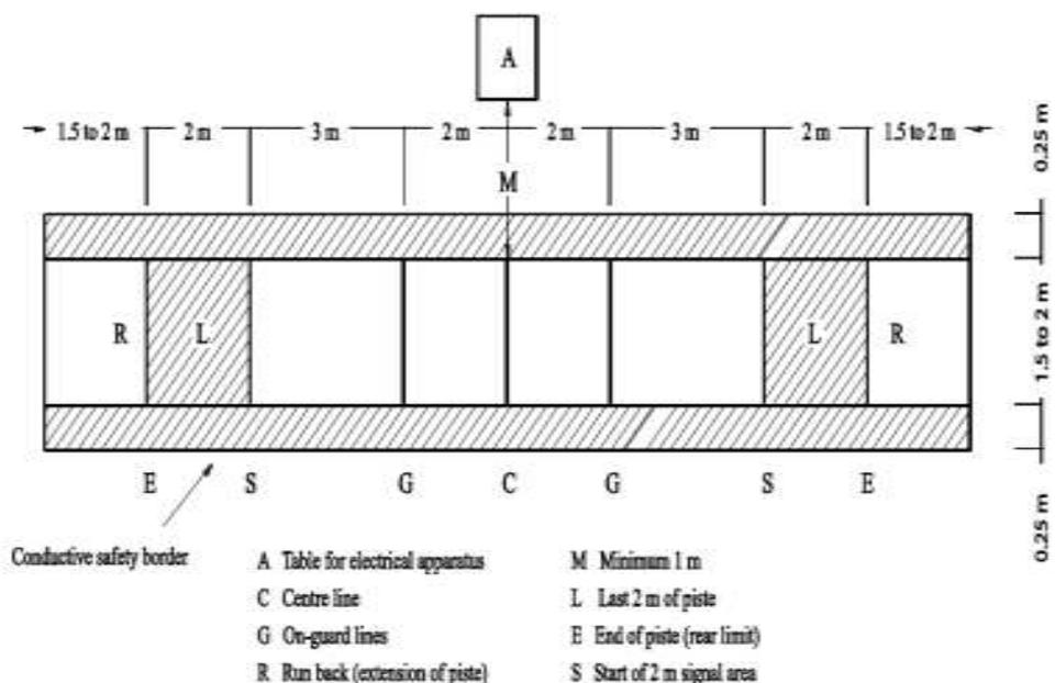
For foil and épée the conductive surface must cover the whole of the length and breadth of the piste, including its extensions (run back) and its safety borders (cf. Article t.13s, m.57)
